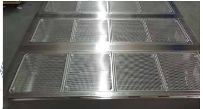
Air supply tower for galley areas
